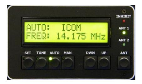
**INHIBIT** Indicates interruption of transmission during the tuning process of the PA. If indicated by RED LED then PA is in STBY mode. If during a retune operations within the same BAND then the PA will retune according to the frequency of
