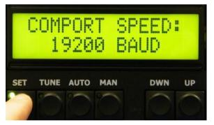
Baud rate for TCVR – PA communication is shown on the LCD display.
