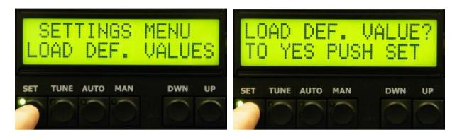
Then select if you want to erase all settings (pressing TUNE) or just one setting value (SET button). In the case of resetting a single parameter use UP / DWN to select which option and confirm by SET.
