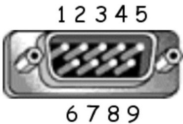
RS232 connection with TCVR. For CAT communication you need connect pin 2 RX-D, pin 3 TX-D and pin 5 GROUND
