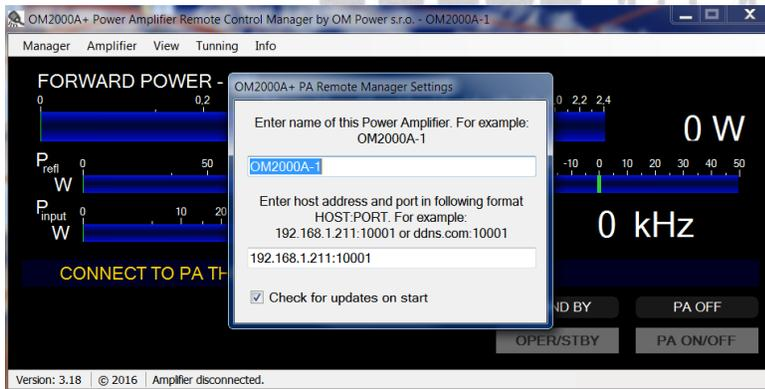
In Remote Control software, open Settings. Enter the IP Address and Port number you set up in previous point in your router. IP Address is the WAN IP Address in basic setup page and Port number is the Port (or Public Port if separate) in forwarding page. When done, click enter.
