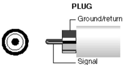
Output signal PTT (maximum switching of 30V / 50mA)
