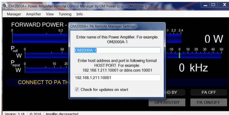
In the Remote Control software open Settings and enter the IP Address and Port number that you set in point 7.5.1.
