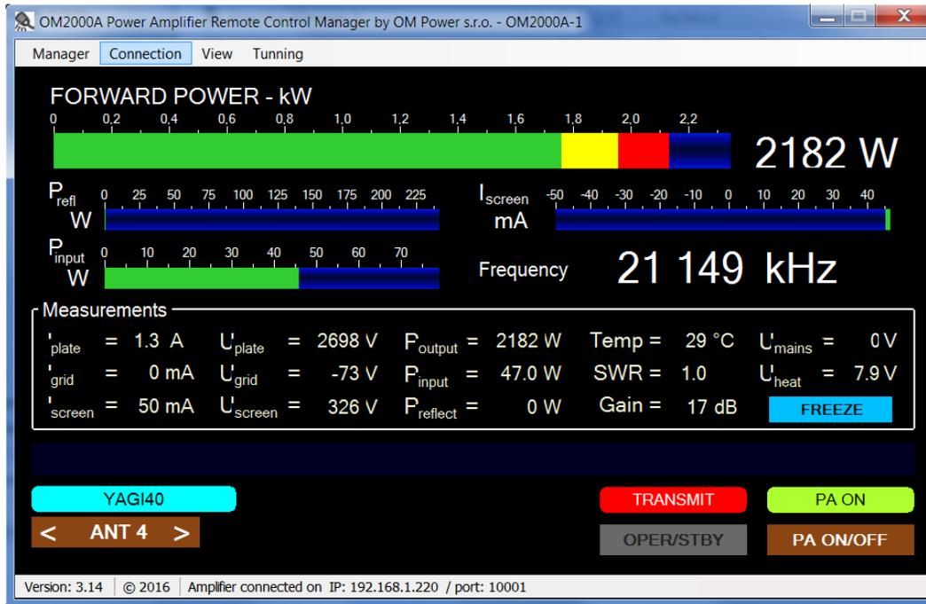
**Fine tune screen.** It is possible to retune the PA remotely (if antenna parameters changed, for example), too. Proceed the same way than with local control (page 28).
