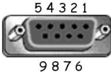
RS232 connection to the computer. For CAT communication you need connect pin 2 TX-D, pin 3 RX-D and pin 5 GROUND
