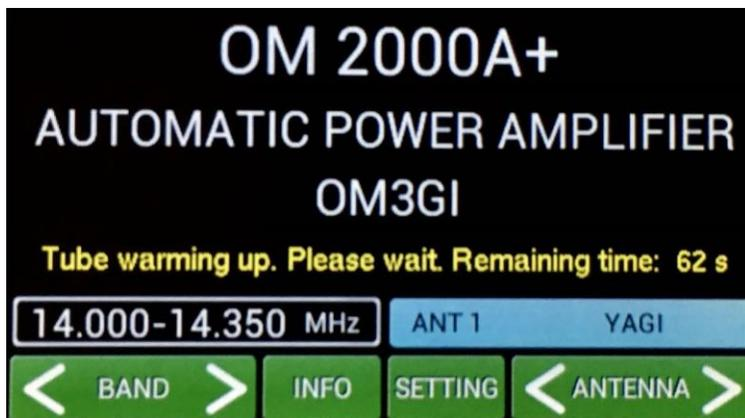
Time to go is visible on the display. Wait until heating finish.
