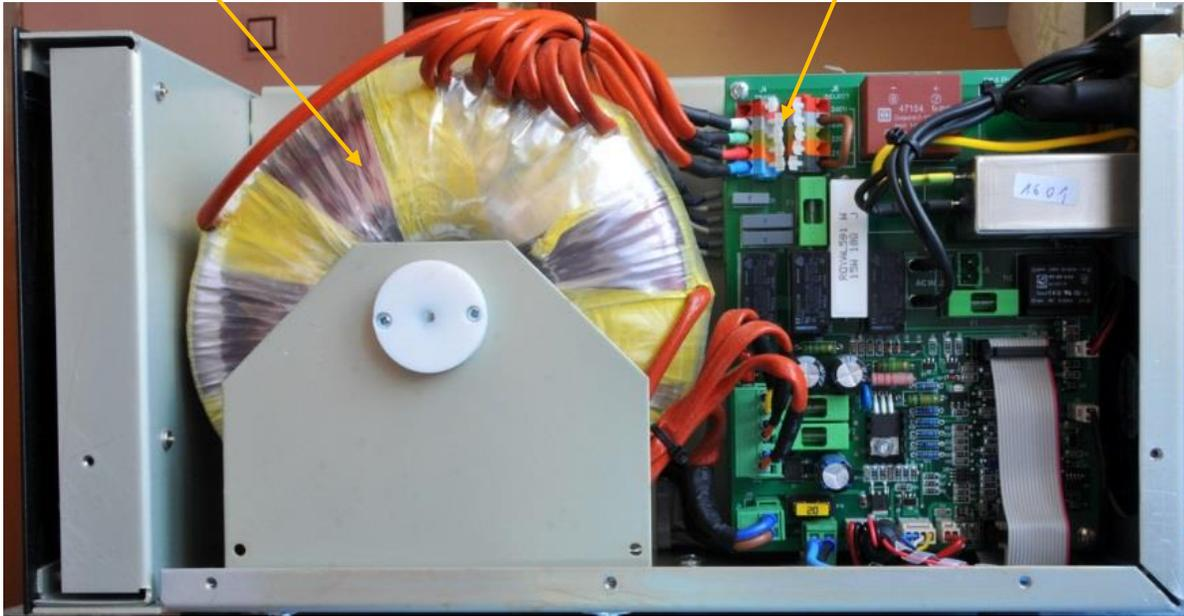
Remove the upper lid first. On the right side of the PA, next to the HV transformer there are two PCBs mounted. On the left upper side of the front (Switch-ON) board connector J6 is located.
