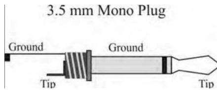
Use CI-V connection for communication with ICOM type transceiver. Signal CI-V is connected to the Tip.
