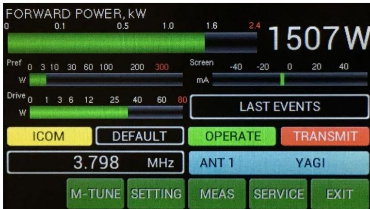
Output power is 1507W, reflected power reached abt. 4W and screen current is abt. -8 mA.
