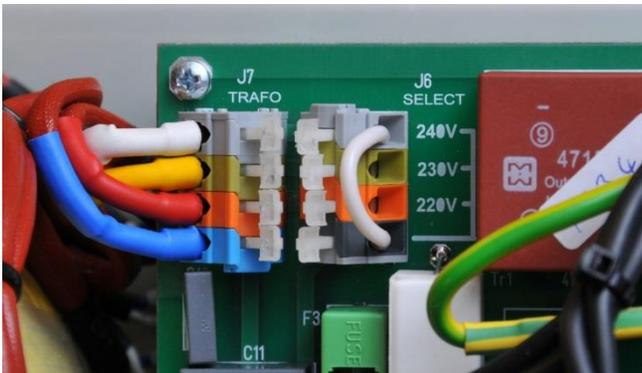
Use flat screwdriver or finger and press carefully the white stick to release contact and move upper end of the white jumper to the proper position, if necessary.
