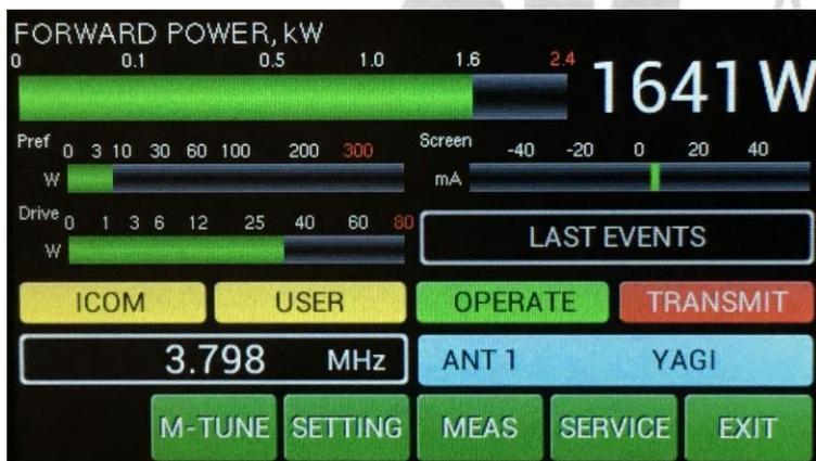
We can see new small yellow window. **USER** means that we used manual tuning feature to optimize the PA adjustment.
