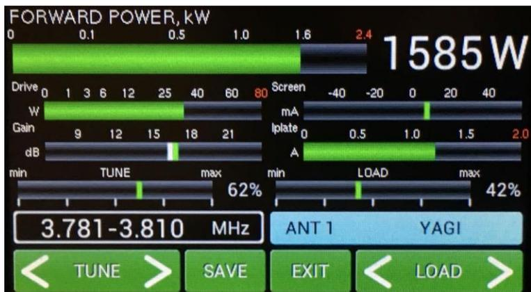
This is the result after manual adjustment process. Output power increased to 1585 W. Screen current is now abt. +10 mA.
