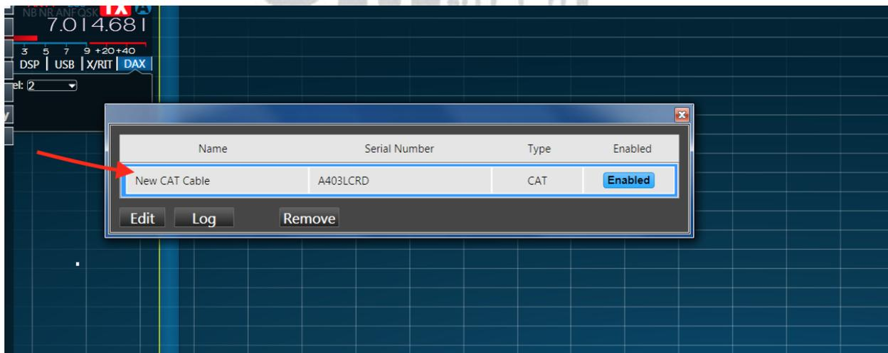
Make double click on the line (with connected USB adapter after that appears possibility) to open configuration window for COM port .
