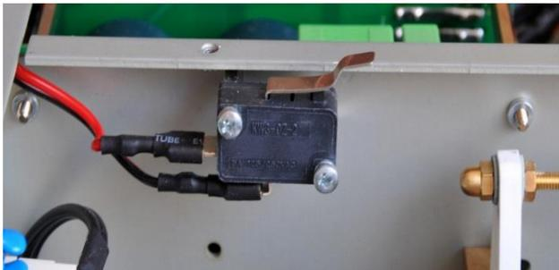
One of the important safety element is mechanical switch for AC blocking at opened amplifier.
