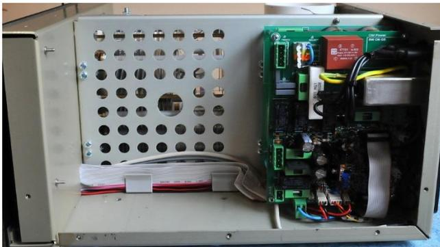
Weight of the PA was distributed (transformer has 12 kg, rest of the PA has cca 12 kg, too).
