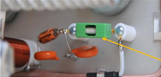
One special fuse filled with sand is used in the model OM2000A+. In the case of an accidental discharges in the tube this fuse (4 Amps fast, filled with sand) saves HV supply circuits.
