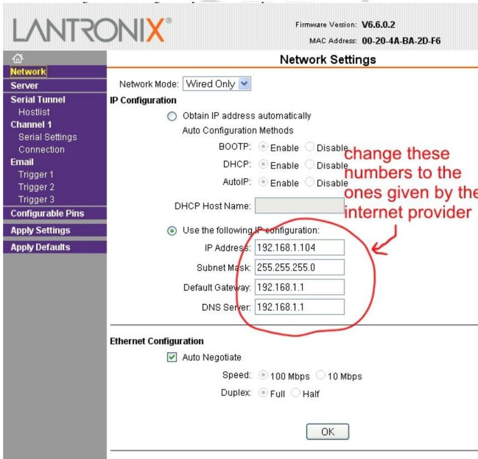
The image shows the LANTRONIX Network Settings page. The page has a header with the LANTRONIX logo, Firmware Version: V6.6.0.2, and MAC Address: 00-20-4A-BA-2D-F6. The main content area is titled "Network Settings" and includes a sidebar on the left with navigation options: Network, Server, Serial Tunnel, Channel 1, Email, Configurable Pins, Apply Settings, and Apply Defaults. The main content area is divided into "IP Configuration" and "Ethernet Configuration".
