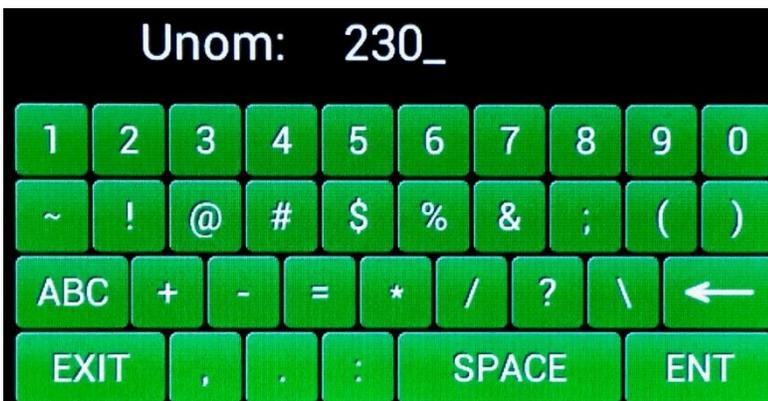
Type proper value of the primary voltage and press **ENT**.
