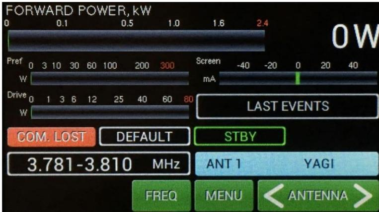
**FREQ** button has two functions. It allows to display working frequency or active band segment.
