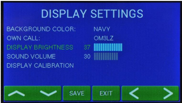
Use next lines and set brightness and sound volume (use up/down and left/right). Confirm with **SAVE**.
