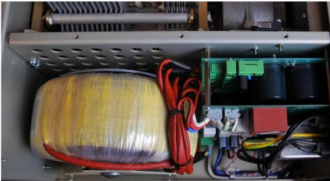
Watch the released terminals, when moving the transformer!
