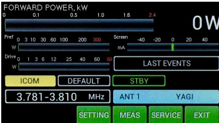
**Menu display** allows to go deeper to the **SETTINGS** mode, **MEAS**uring mode or to **SERVICE** mode.
