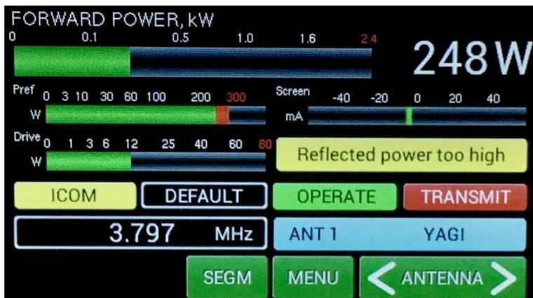
This an example from previous attempt, when antenna was disconnected from the PA during transmitting.
