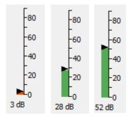
I suspect the WSJT-X bar graph was modelled on Star Trek's medical bay © The bar graph bar should normally be green, showing acceptable levels. If it is red, the level is probably too high (causing distortion, apparently wide signals and poor copy) or too low (no input, no signals to copy!).
