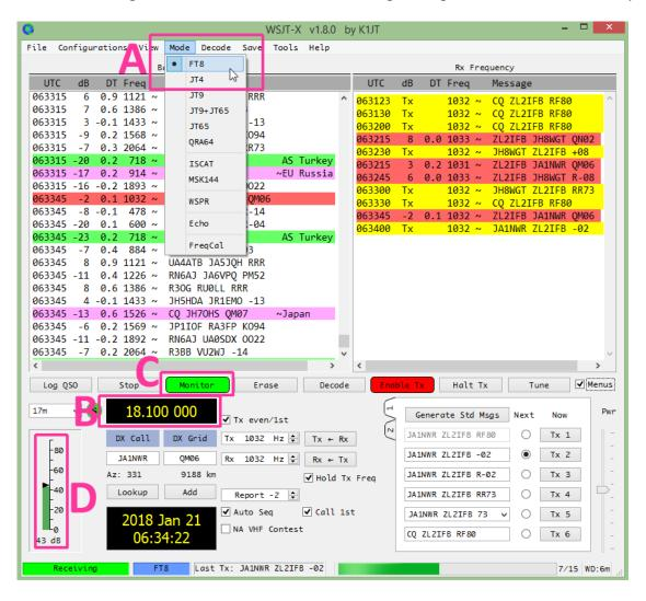
Do you see a smattering of yellow and red blobs on the waterfall? Is the rig on the right mode and antenna? Can you hear the weeeeee of FT8 signals on your receiver? Is the rig on? FT8 is a *weak-signal*, not a *no-signal* mode!
